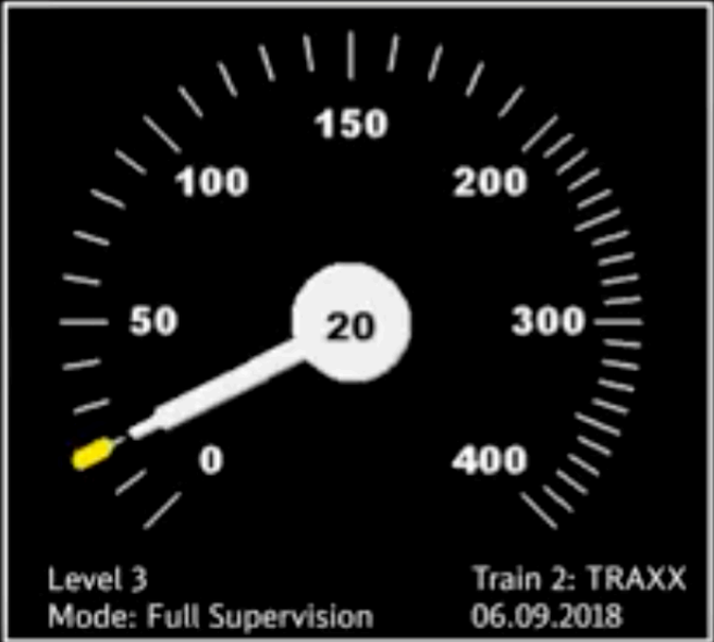
Train 2 following Train 1 (Lucy) on the same occupied track section but on different virtual subsections
